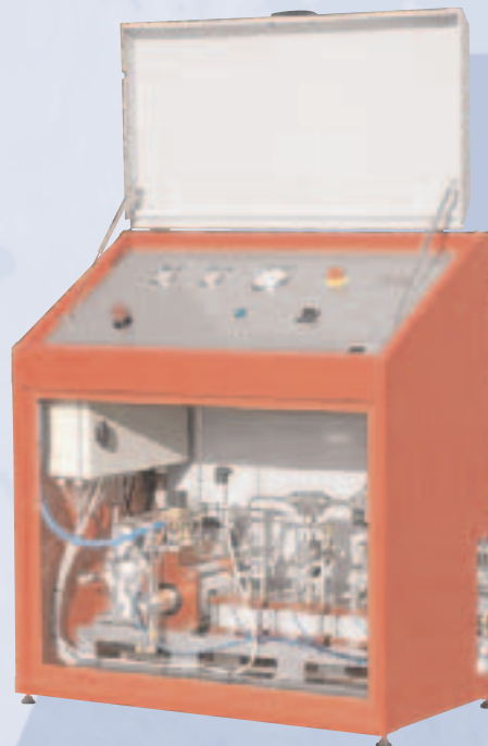
Workshop test unit HPU for hydroforming
